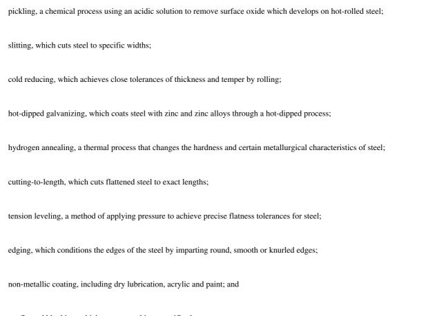
configured blanking, which stamps steel into specific shapes;
